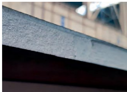
Figure 1: Detail of the overlapping of two subsequent cuts of side trimming shear, showing a perfectly straight edge.
