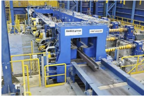
Figure 4: Largest CRS-Roller Straightening Machine (CRS 2800)
