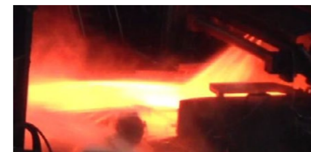
Figure 3: Scale breaker causes huge water and steam load
