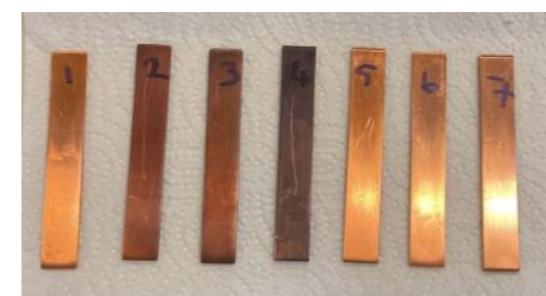
Figure 18. Copper strip corrosion test results
