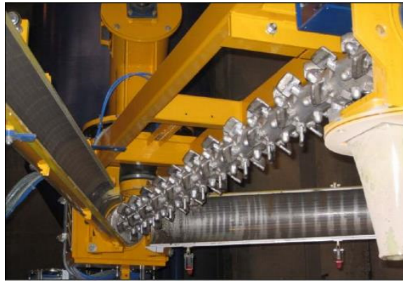
Figure 10. ANKERTUN CS mixing shaft and opened housing [4].
