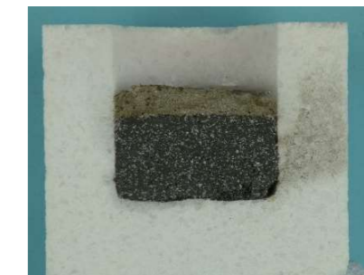
Figure 7: 2 C-Crucible Test with well filler and ladle slag after 1100°C/2h in oxidizing atmosphere
