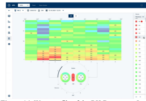
Figure 14. Wear profile of the RH Degasser – Lower Vessel
