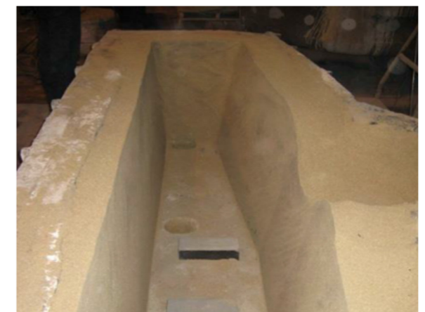
Figure 9. Tundish after removing the template. [5]
