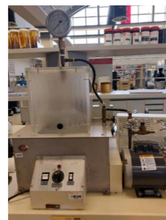
Figure 5. Water spray test device
