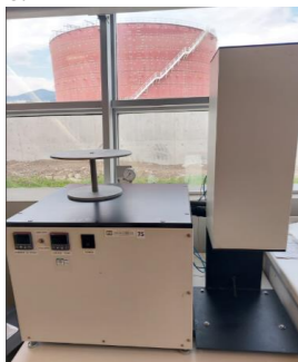
Figure 8. Grease mobility test device
