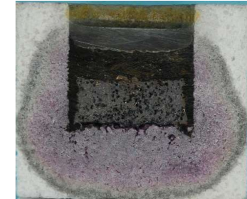
Figure 13: 2 C-Crucible Test with well filler and crude steel after 1600°C/2h in reducing atmosphere
