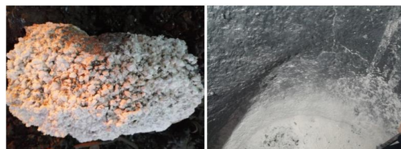
Figure 3. Image of induction furnace where wear is not homogeneous due to non-uniform grain distribution.
