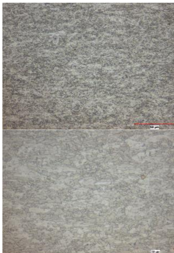
Figure 6: S700MC microstructure X-200 and X-500
