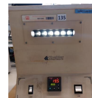
Figure 7. Dropping point test device
