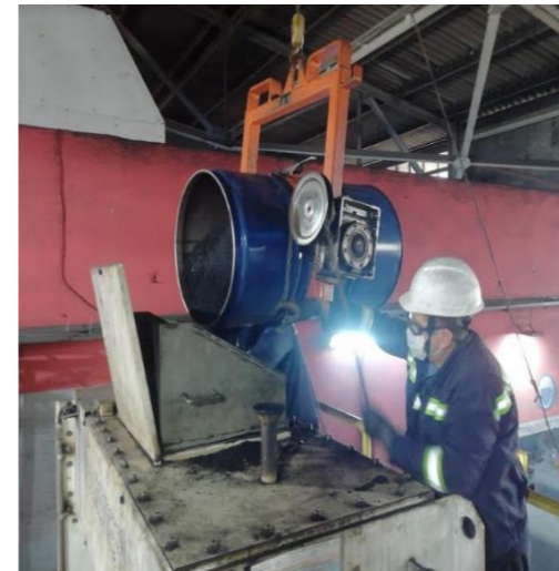
Figure 7. Mixing of coal and waste materials in the mixer.
