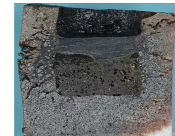
Figure 12: 3 C-Crucible Test with well filler, ladle slag, crude steel after 1600°C/2h in oxidizing atmosphere
