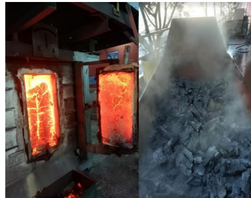
Figure 8. The coking oven and the coke obtained
