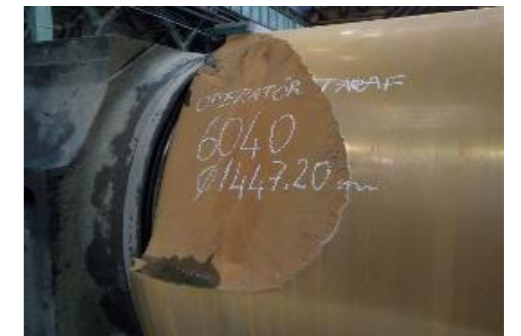
Figure 3. Backup roll spalling
