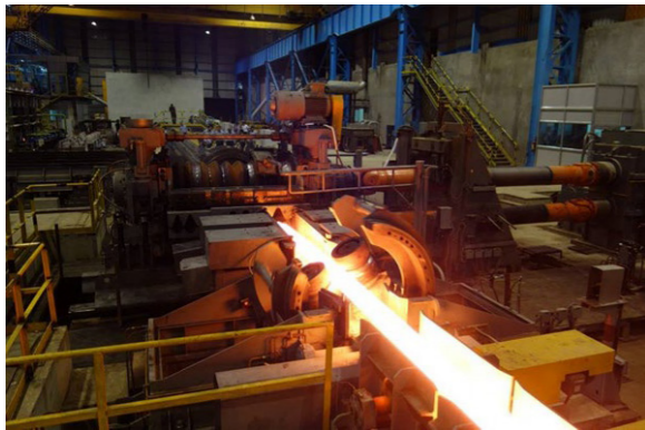
Figure 2. Reversing sliding breakdown with bar rotating.
