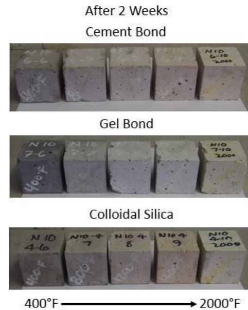
Figure 9. Samples after being removed from acid bath.
