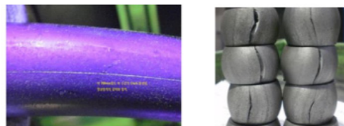
Figure 3. Destructive verification of very fine seam cracks detected inline by imaging technology.
