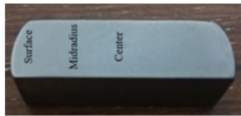
Figure 4. Cross-section of a typical specimen showing the 3 different locations where metallographic examinations of TMR and CR processed rods were conducted.
