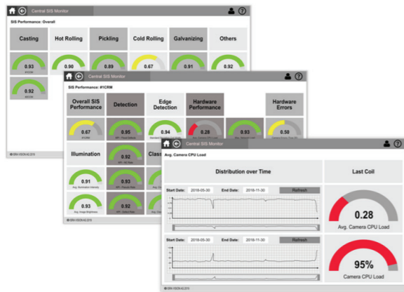
Figure 7. Drill-Down from single SIS performance KPI to underlying KPI with its history
