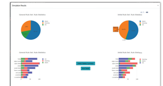
Figure 6. The simulation of the new rule set shows the percentage OK material and the rule(s) causing blocking
