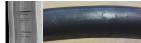
Figure 14. Rolled in scale (left: inline image; right: rod sample).
