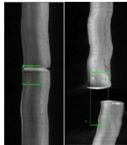
Figure 12. Left: Necking of a 5.5 mm wire at 105 m/s; Right: Wire Break.
