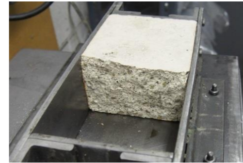
Figure 4: Substrate positioned in mold
