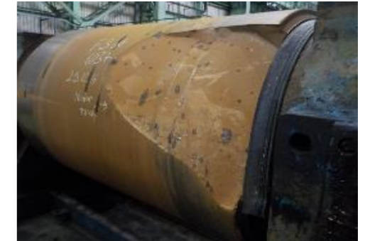
Figure 2. Backup roll spalling
