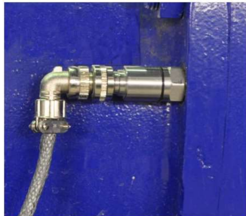
Figure 2. Prüftechnik VIB 6.172 accelerometer installed on the bearings
