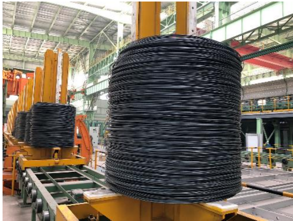
Figure 12. Vertical pallet coil handling system.
