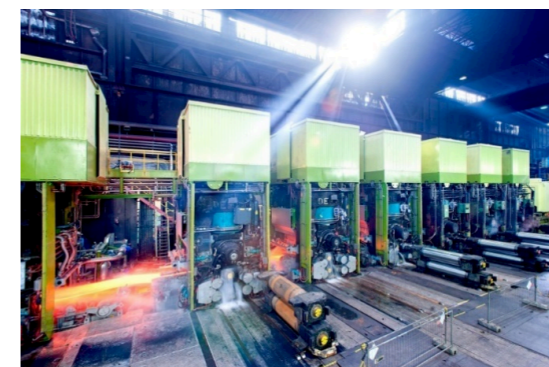
Figure 1: HSM - finishing mill section
