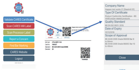
Figure 4. Scanning CARES Approved Company static QR code
