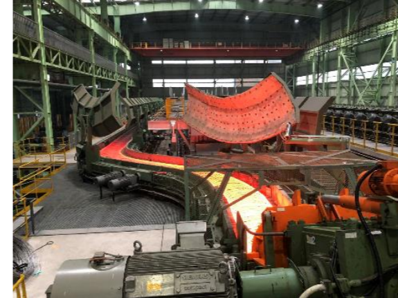
Figure 9. Morgan Stelmor Conveyor and DST line.
