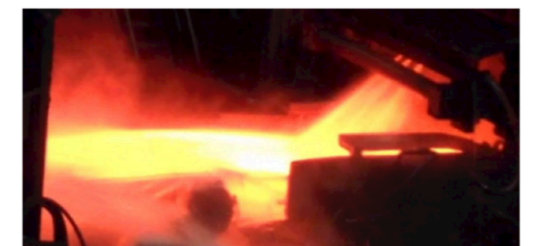
Figure 3: Scale breaker causes huge water and steam load
