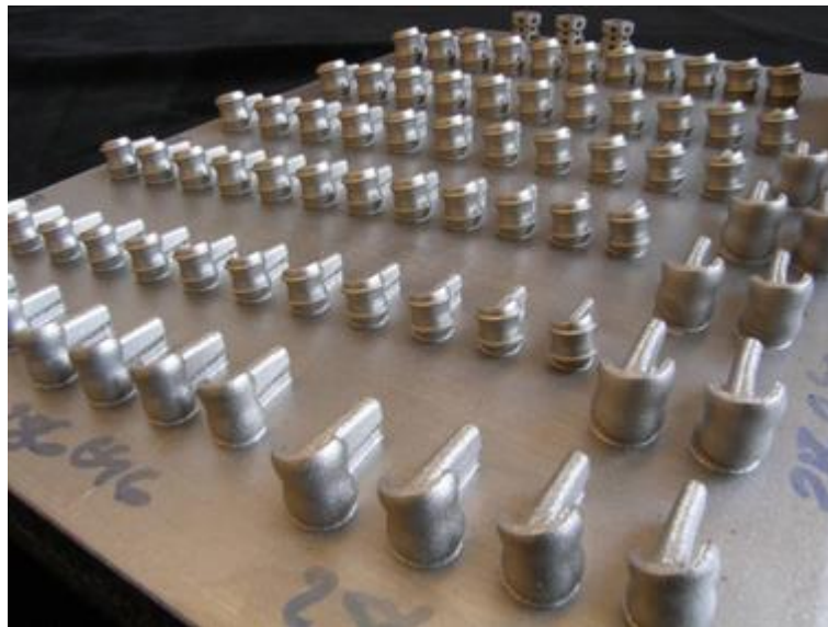
Figure 7 Batch of finger implants in EOS CobaltChrome MP1 [2].
