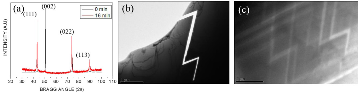
Figure4. (a) XRD Patterns from the sample S0 and S16. (b) The transgranularly propagated cracks observed on the sample S8. (c) Step-like crystallographic defects from the sample S0.
