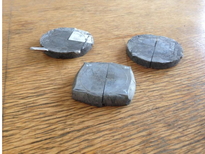
Figure 4. Produced disks after T6 heat treatment.
