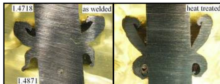
Figure 3. Cross-sectional macrophotographs of as-welded and heat treated joints
