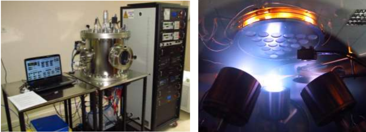
Figure 1. a) Thin film deposition system and b) viewgraph showing three targets and the magazine older incorporating 21 glass substrates.
