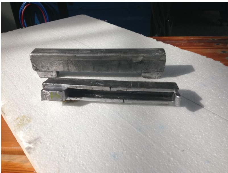
Figure 5. Produced hollow shaped parts after T6 heat treatment.
