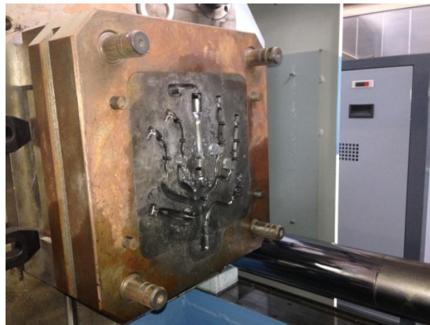
Figure 7. The die mold that can produce tensile test specimen and bending test specimen.
