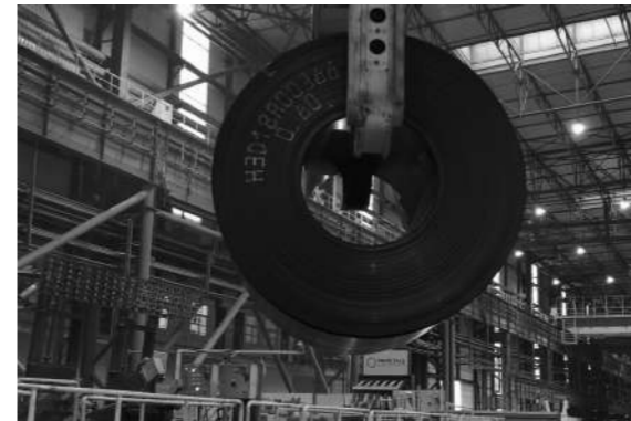
Figure 1 Arvedi ESP mill produced ultra-thin hot strip with a thickness of 0.6 millimeter
