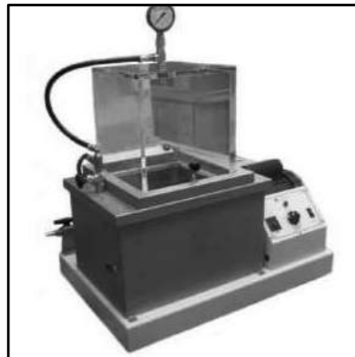
Figure 5: ASTM D 4049 – Device of Amount of Sweeping of Greases from Surface by Water Spray Method
