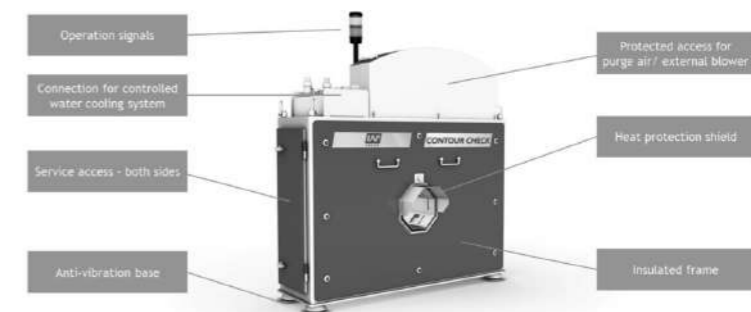
Fig. 8 –Measurement Gauge of the CONTOUR CHECK SHAPE for Dimensional Measurement of Long Products
