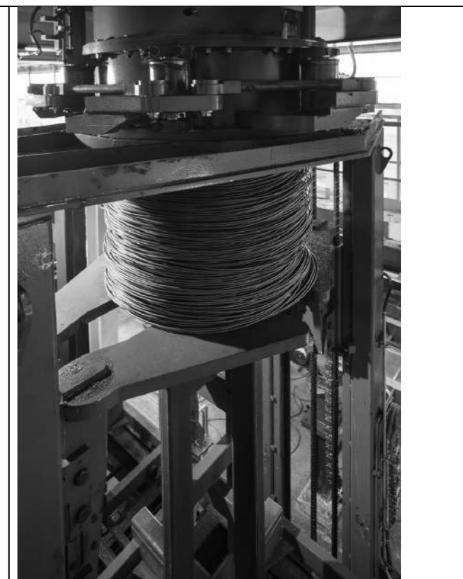
Figure 11: Coil formed and laid down on coil lowering station
