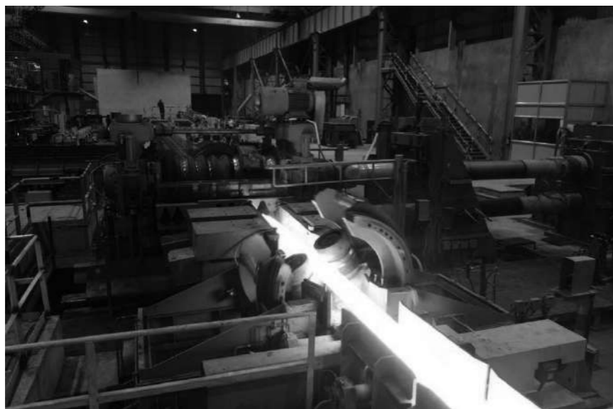
Figure 2 – Reversing sliding breakdown with bar rotating device
