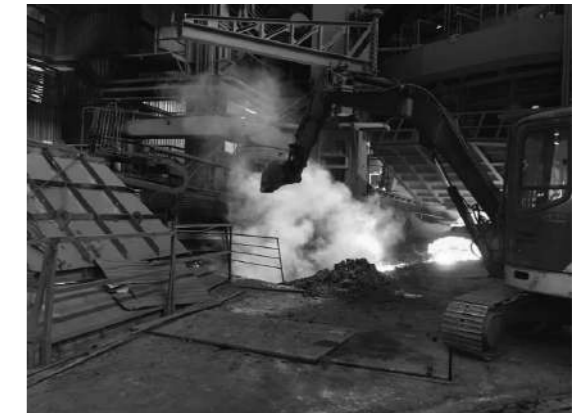
Figure 7. Addition of ladle furnace slag during the pouring of hot metal in blast furnace.
