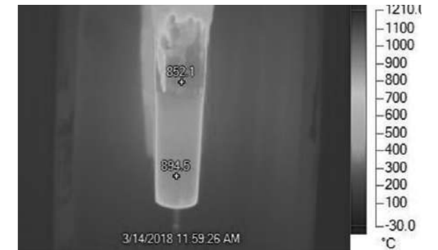
Figure 6: Thermographic image of tube during preheating.
