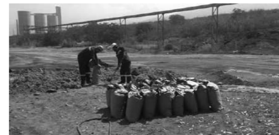
Figure 6. Packaging the ladle furnace slag with paper bags.
