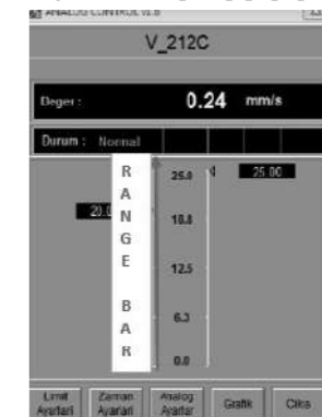
Figure 3: The pump popup on the scada system
