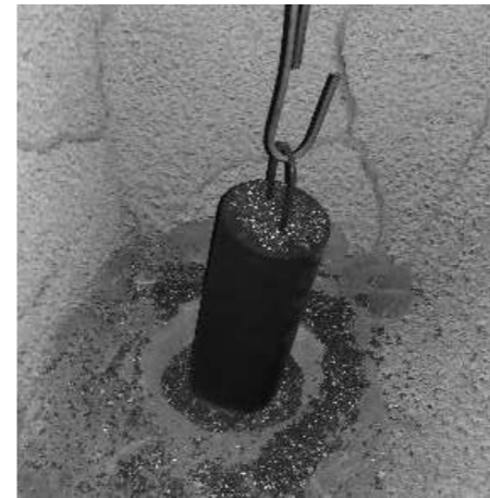
Figure 5: Third starter tube, with 240mm height, closed top with swarf setting.
