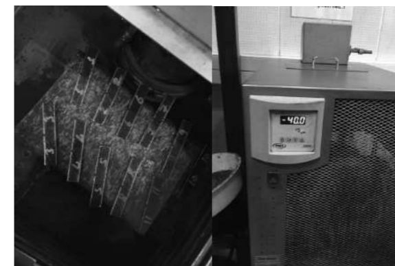
Figure 7. Impact Test Specimen at Cooler
