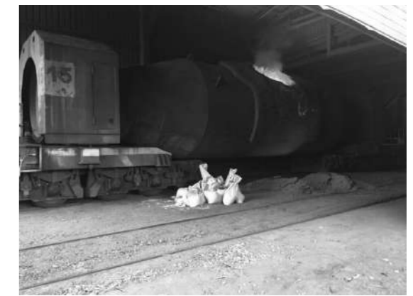
Figure 8. Addition of LF slag at hot metal pit into the runner.
