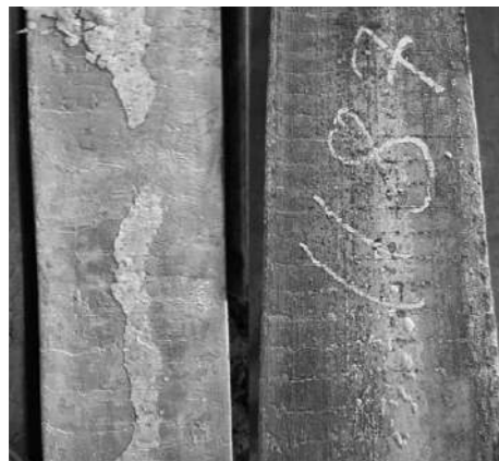
Figure 10: Comparison of a regular billet cast with opened stream (strand 1 – left) and a billet cast with CNC Shrouded with flux powder (strand 6 – right).
