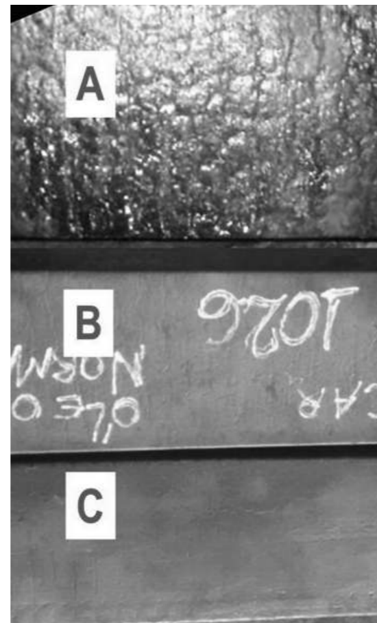
Figure 11: Samples of billets after blasting. Sample A was the standard open stream with oil (strand 1), Sample B was from trial number 5, cast with the shroud and oil as lubricant, and Sample C was from trial number 6, cast with the shroud and flux powder as lubricant.
