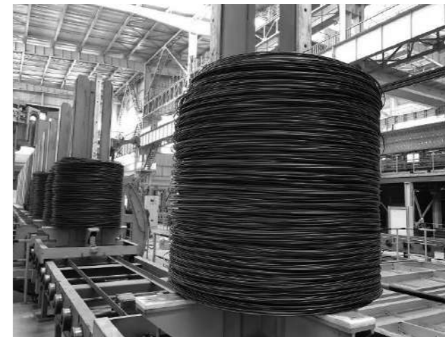
Figure 12 – Vertical pallet coil handling system
