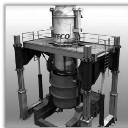
Figure 4 Hydraulic lifting system
