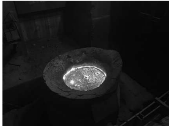
Figure 9. The conditions of slag after LF slag addition in hot metal pit.
