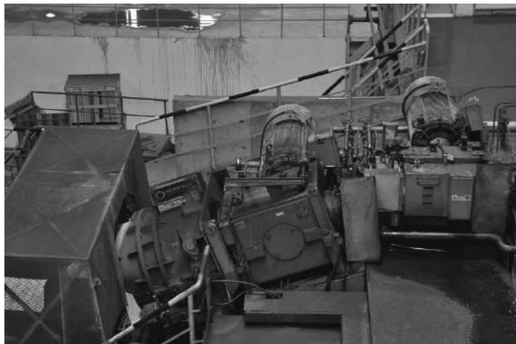
Figure 8 – Morgan High Speed Laying Head and Pinch Roll
